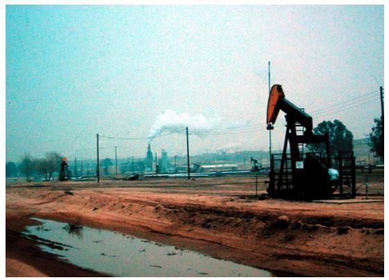
**Figure 5.** Secondary recovery is used in most oil fields to enhance production. Water is injected commonly and is used in Saudi Arabian fields, while steam shown here is used too. The steam plants, shown in the distance venting steam, pump steam into the oil-bearing strata and force the oil to other wells nearby where it is extracted. The technique works on heavy crude and fields that are somewhat depleted. See http://www.heavyoilinfo.com/thermal . J. H. Lipps image, 1960.
