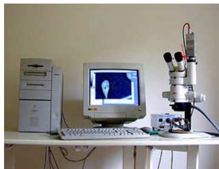
Figure 1. 1. Imaging station used for the present study. See Figure 1B for digital dial gauge, which is mounted on the back side of the binocular microscope (red arrow) and allows the user to measure the vertical displacement of the lens-system during focusing. 1.2. Digital dial gauge to measure the vertical displacement of the lens-system during focusing. The arrow points to the contact between the fixed part of the stand (black) and the moving part of the binocular microscope (white).
