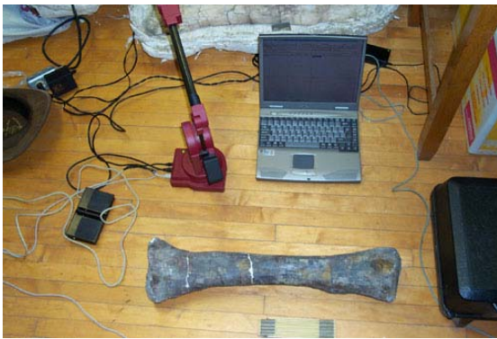
Figure 1. Microscribe digitizer connected to a notebook computer and ready to collect data.
