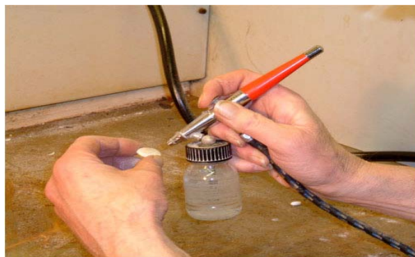
Figure 7. The Paasche airbrush, suitable for small-scale wetblasting.
