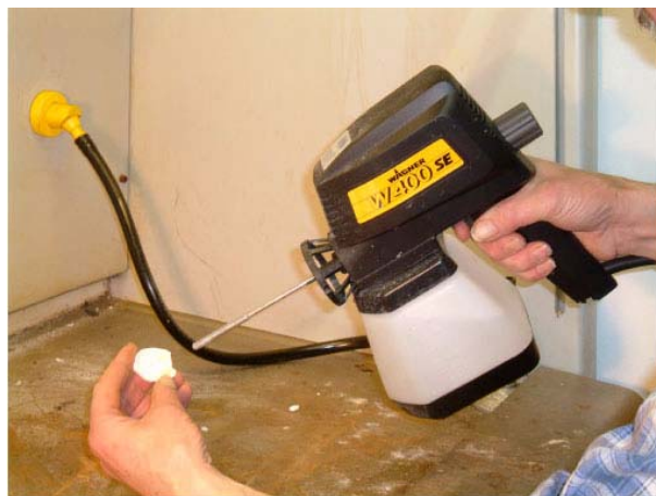
Figure 3. The Wagner watergun, suitable for medium-scale waterblasting.
