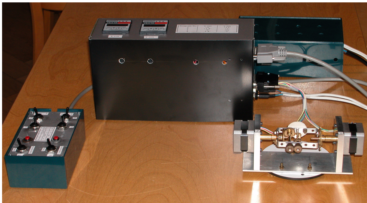
Figure 6. Components of the XY-tilting stage. The large box in the center of the image contains the two programmable Vexta controllers for the X- and Y-axes stepping motors. This component can be connected to the PC for controlling of the motors via software. Alternatively, it can be connected to the logic switch-box for manual control of the motors (small blue box to the left side of the image). This second combination is entirely independent from any computer and makes the stage portable. The switch-box allows the user to select between forward/backward and slow/fast movement of the motors. When pressing the red contact switches, motors move by a selected number of steps. The blue box in the background contains the power supply.
