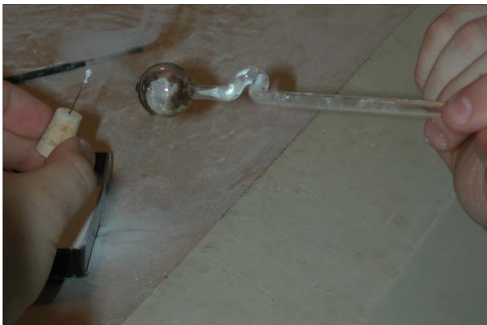
Figure 4. Coating a specimen with ammonium chloride ( \text{NH}_4\text{Cl} ). The compound is heated and vaporized in a glass instrument and then mouth-blown onto the surface of the specimen.
