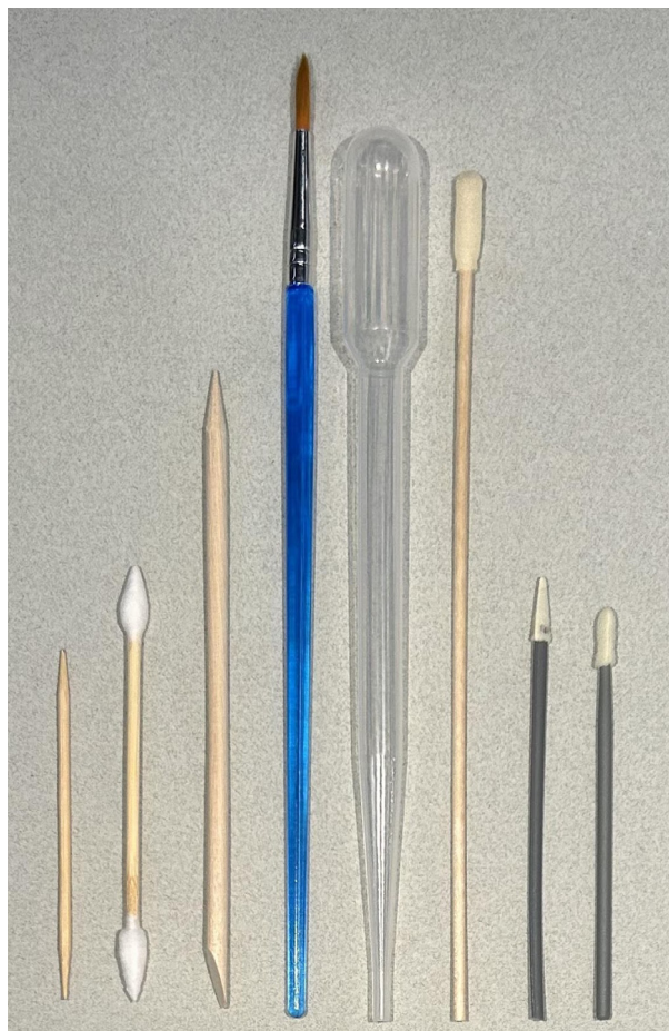
FIGURE 5. Hand tools used in preparation, from left to right: bamboo toothpicks, double tipped cotton swabs, wood manicure sticks, synthetic filament paint brushes, polyethylene bulb droppers, and polyurethane foam swabs.
