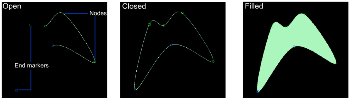
Figure 18. Curve modes. Note that in Open mode curves have two square end markers, which are specialised nodes through which the curves does not pass, but whose position affects the curvature of the final section. The blue square affects the end with the blue circle, the green square the end with the green circle. When the curve is closed these are treated as normal nodes.
